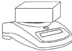
Keep the balance clean. Do not stack material on the balance / balance pan when it is not in use. The Compact balance has a stacking feature for stacking more than one unit on top of each other, which does not apply weight to the pan. For more details on this, see the section on storing
