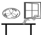
Do not place near open windows, air-conditioning vents or fans that may cause a draft and unstable readings.
